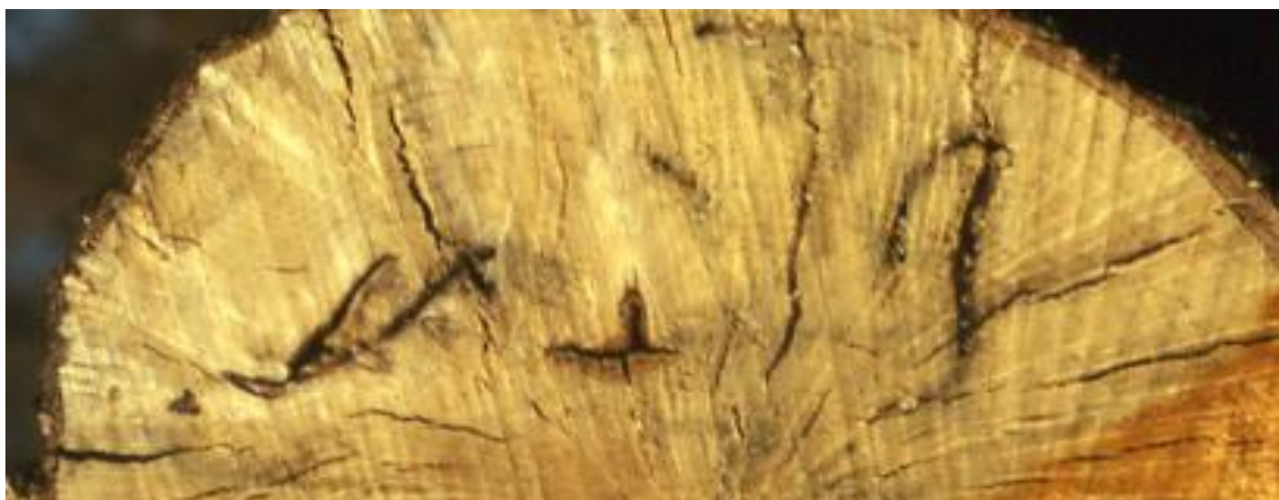
Figure 16: Channels bored by the Ambrosia Beetle Source: DISAFA Entomology, University of Torino
